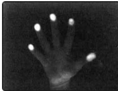
Figure 8: Image showing blob detection from an infrared camera on a multi-touch device (Natural User Interface Group, 2009, "Multi-Touch Terminology").
