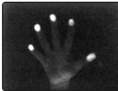
Figure 1: Screen capture of a hand from an infrared camera using the FTIR method. (Natural User Interface Group, 2008b)
